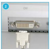
**DVI port (Source : Digital)** : Connect the DVI cable to the DVI port on the back of your monitor.
